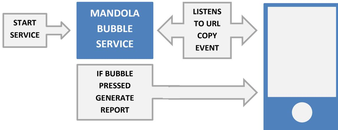
Figure 9: Smartphone app Bubble module diagram.
